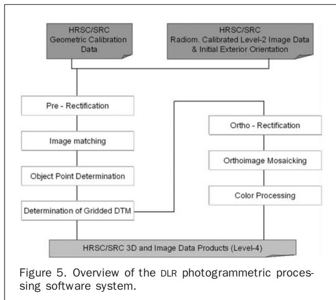
Figure 5. Overview of the DLR photogrammetric processing software system.
