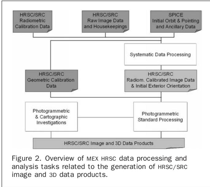
Figure 2. Overview of MEX HRSC data processing and analysis tasks related to the generation of HRSC/SRC image and 3D data products.
